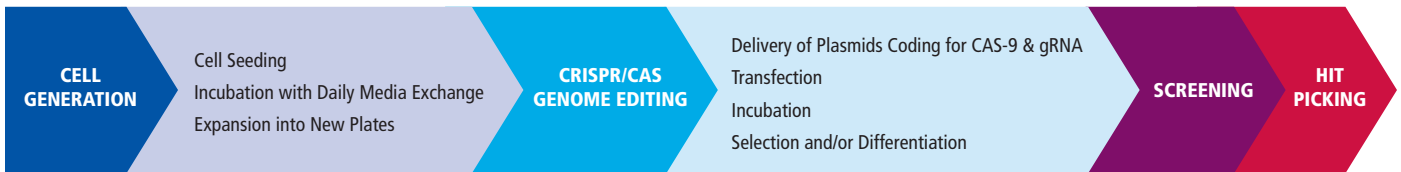
Figure 3. explorer™ workstation workflow for iPS cells and CRISPR.
